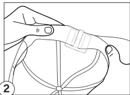
3. Mount the device over the hat, pressing the tabs into the slots.
